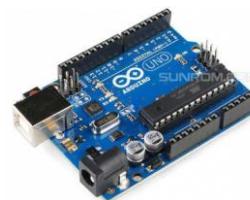
Fig.2 Shows Arduino Development Board
