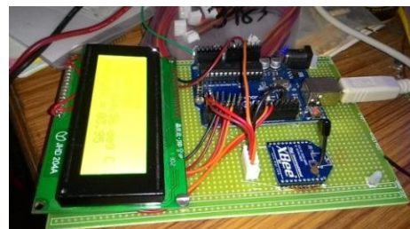
Fig. 9 shows the receiver and display node
